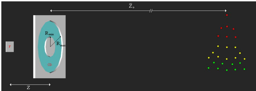
**Figure 1:** Experimental setup to the image caption.  $Z$  is the distance between the film and the CD.  $\bar{Z}_o$  is the distance between the object and the CD.  $R_{\min}$  and  $R_{\max}$  are the minimum and maximum radius of the CD.
