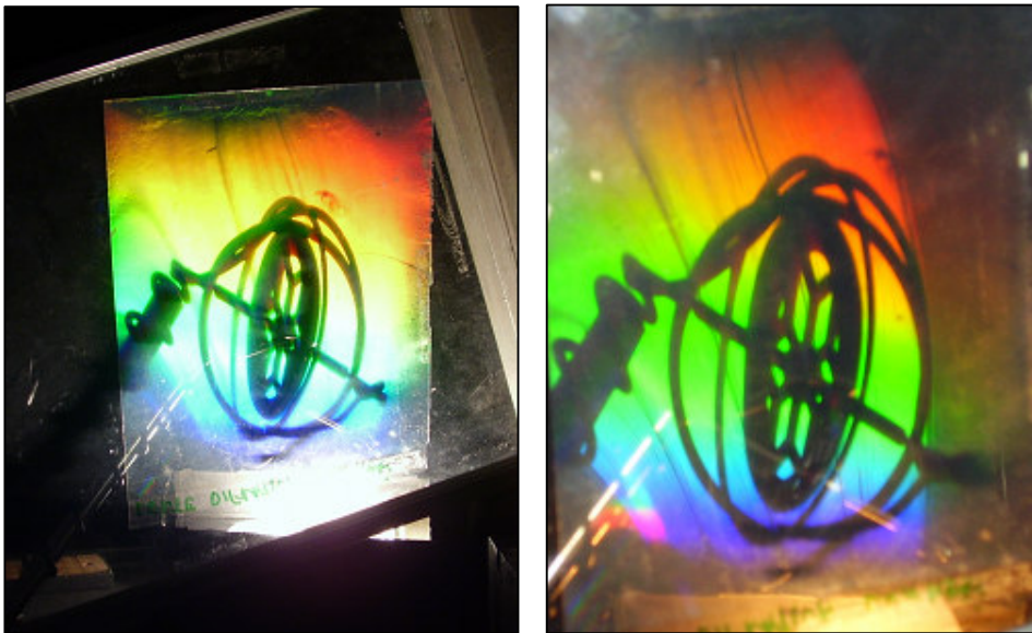
Figure 6: 3D shadowgram of a 3D object, left: observer is located more far of the diffractive screen that in the right image.
