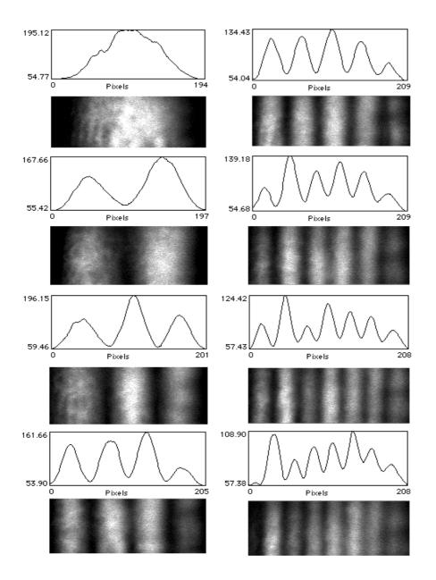
**Figure 2** Dynamic Moiré patterns produced by two sinusoidal phase grating superposition. According to Eq(9), in the left column, up to down the j = 1,2,3 and 4. In the right column, up to down the j = 5,6,7 and 8.
