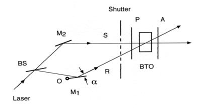
Figure 1: Experimental setup sketch. The mirror M1 is electronically controlled to produce small rotations around point O.
