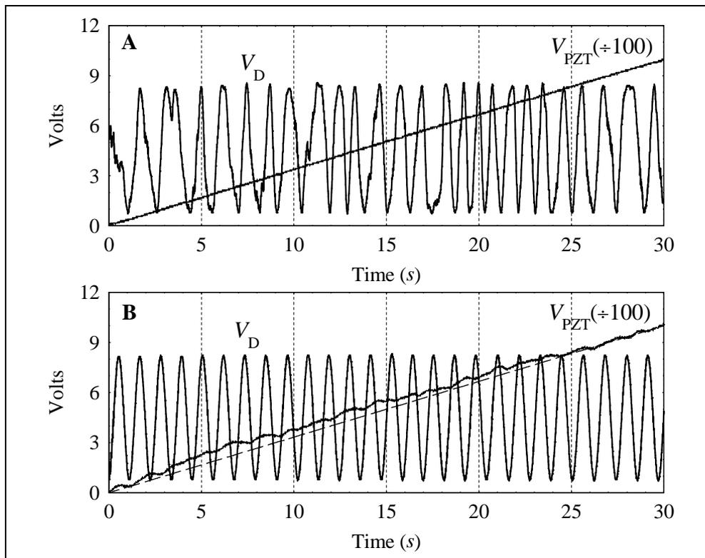
**Figure 2:** Experimental results, comparing the movement of the optical fringes with and without feedback.  $V_D$  is the output voltage of the photodetector and  $V_{PZT}$  is the voltage applied to the piezoelectric actuator (divided by 100). In Fig.2A, the interferometer operates in open loop (without feedback), whereas in Fig.2B the error signal is fed back to the interferometer.
