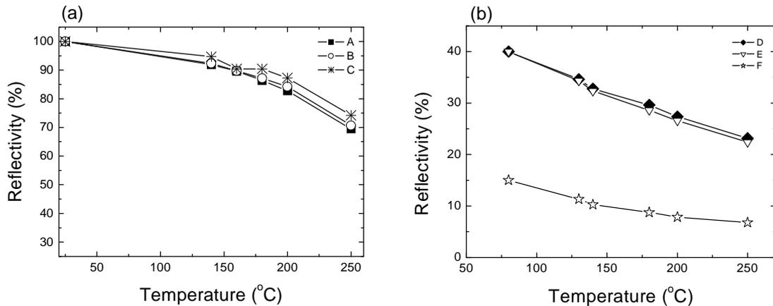
**Figure 2:** Reflectivities as a function of treatment temperature for the FBG: (a) recorded with pulsed laser; (b) recorded through cw laser exposure.
