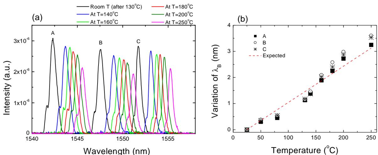
**Figure 1:** (a) Reflectivity spectra, at high temperatures, for the FBG recorded with pulsed laser; (b) variation of the Bragg wavelengths at high temperature: points are experimental data and the dotted line is the theoretical curve.
