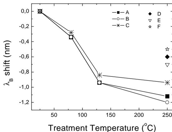
**Figure 3:** Bragg wavelength shifts, measured at room temperature, after thermal treatment at the indicated temperatures. Lines plus symbols: FBG recorded with pulsed laser. Symbols: FBG obtained and through cw laser exposure.
