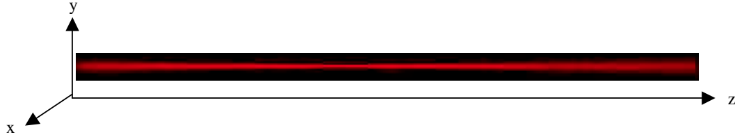
Figure 2: Digital image of the scattered laser beam ( y : 32 pixel; z : 880 pixel).
