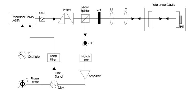
**Figura 1**. Experimental setup of frequency stabilization for a diode laser, using an active locking technique to the Fabry-Perot cavity, by the Pound-Drever-Hall error signal. O.D. = Diode optical, DBM = double-balanced mixer.
