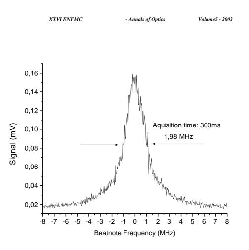
**Figura 2:** Beatnote signal between the two stabilized diode lasers, locked independently to resonance of two Fabry-Perot cavities by the Pound-Drever-Hall technique.
